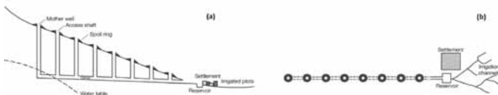
Figure 19. Typical cross section and bird view of a karez system (Source: Kamaz, Z. 2010)
