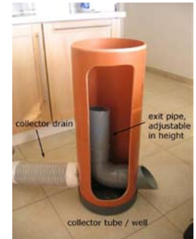
Figure 2: Collector tube well
