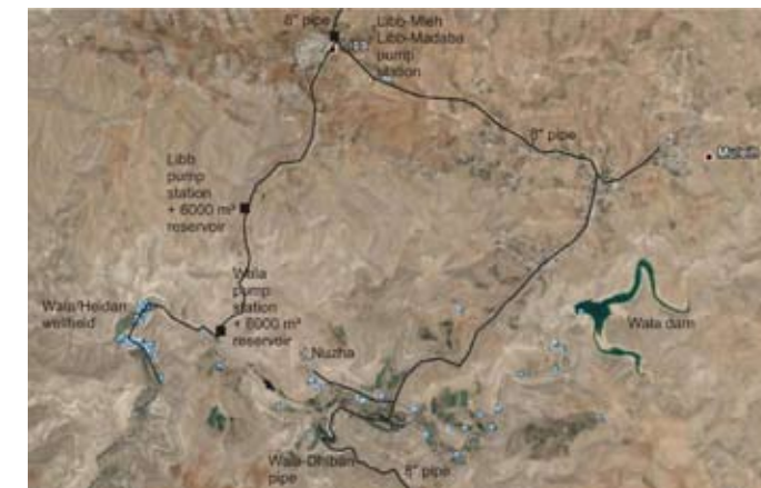
Figure 5: Locations of Wadi Wala Dam and Wala/Heidan Well Field with Water Supply Network (the green areas between the reservoir and the well field indicate irrigated areas)
