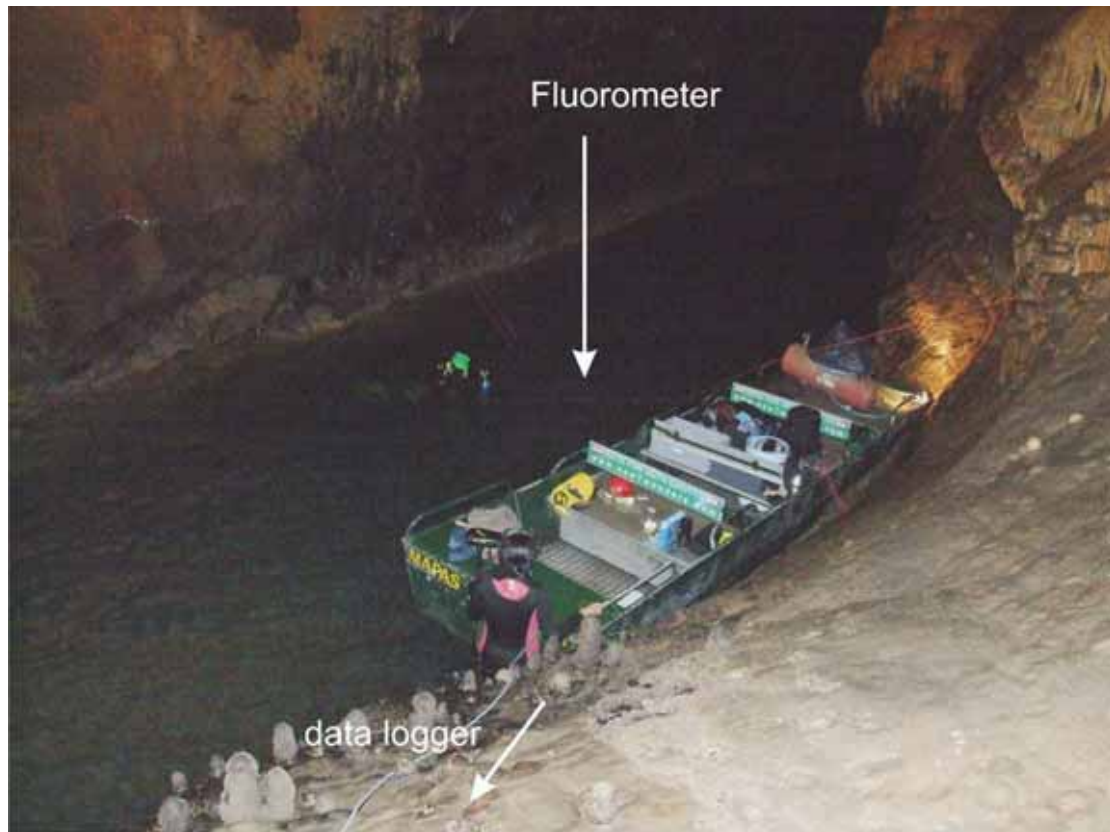
Figure 25: Monitoring of tracers at monitoring site 2 (Jeita Grotto) with mobile Albillia fluorometer GGUN FL30
