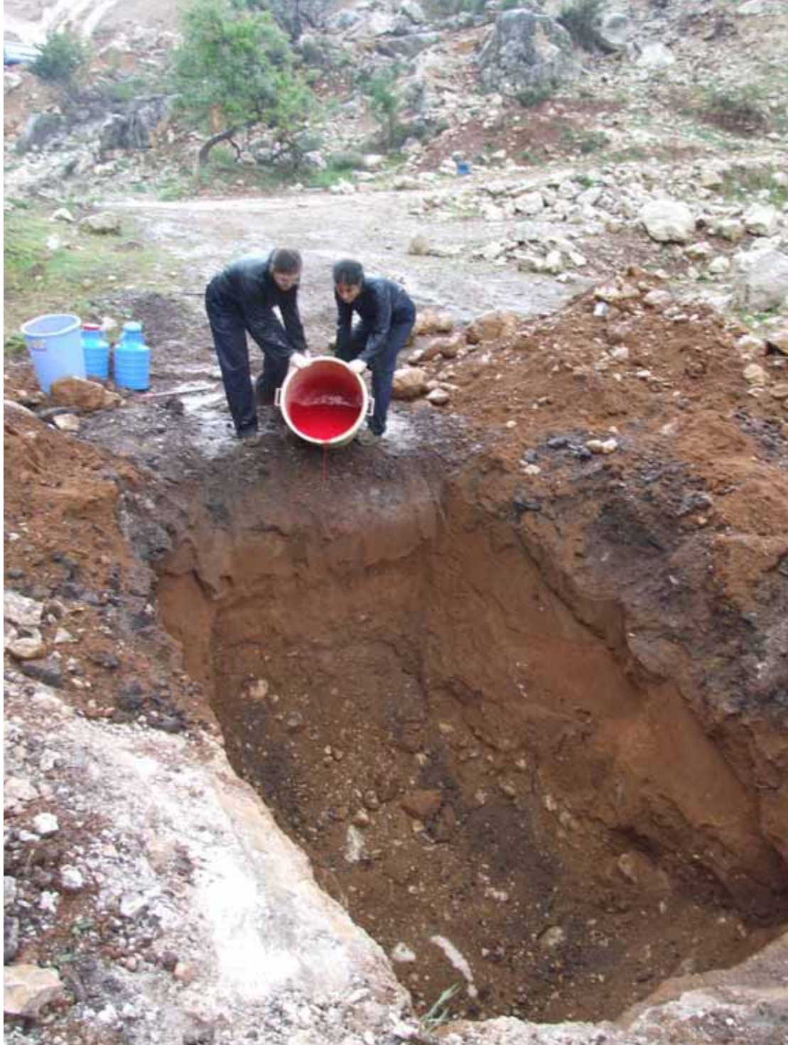
Figure 21: Injection site 2, Test 1A-2 (during injection of amidorhodamine G)
