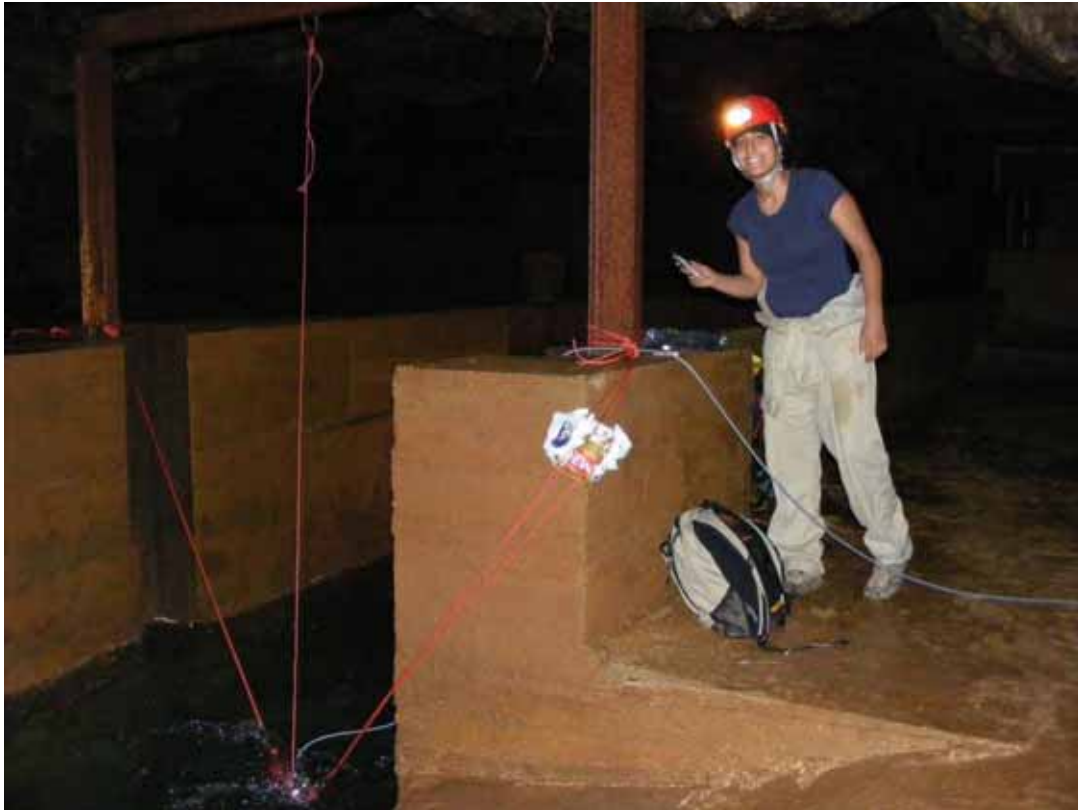
Figure 24: Monitoring of tracers at monitoring site 1 (siphon terminal / Daraya tunnel) with mobile Albillia fluorometer GGUN FL30
