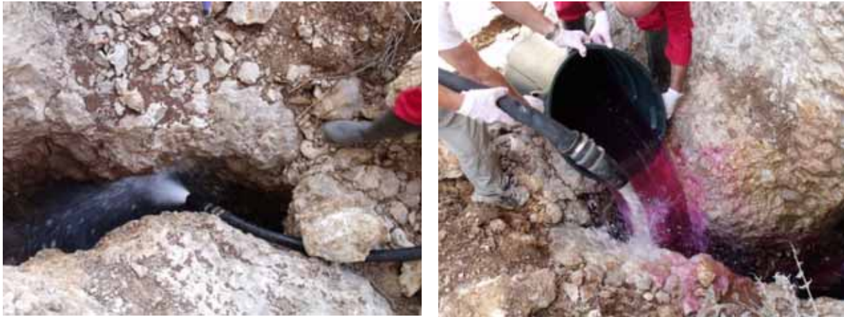
Figure 2-3 Injection of 5 kg of Na-Naphtionate and Amidorhodamine G into the sinkhole “Ras el Astar” in New Ajaltoun
