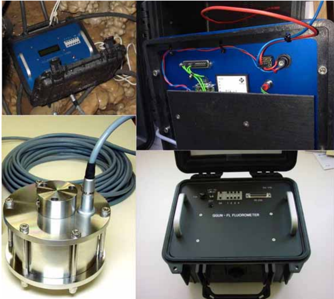
Figure 23: Albilia GGUN FL30 fluorometer used for detection of tracers
