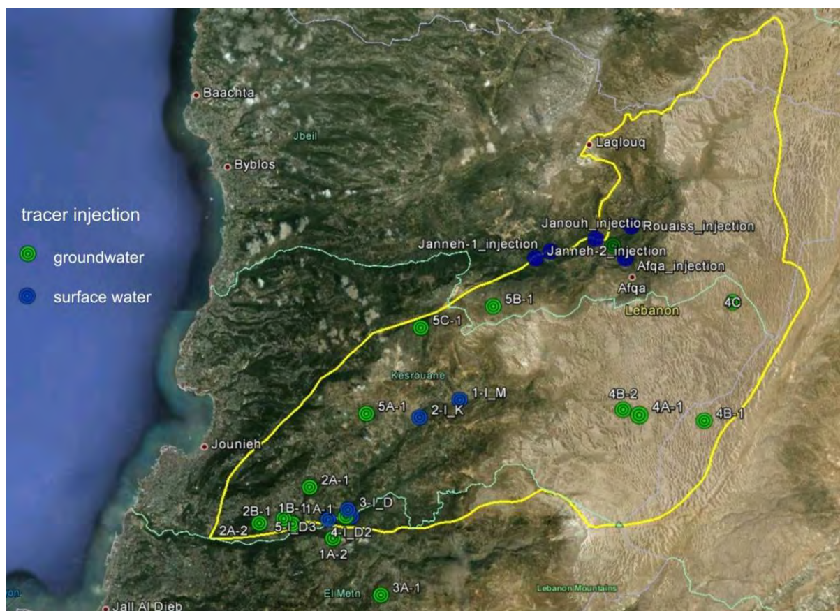
Figure 7: Boundary of Jeita groundwater catchment based on tracer tests (remark: numbers refer to tracer tests documented in MARGANE et al., 2013)
