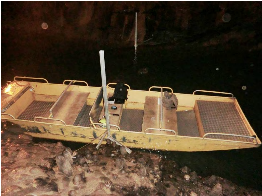
Figure 48: Aluminum frame for measurement of flow-through profile at ADCP
