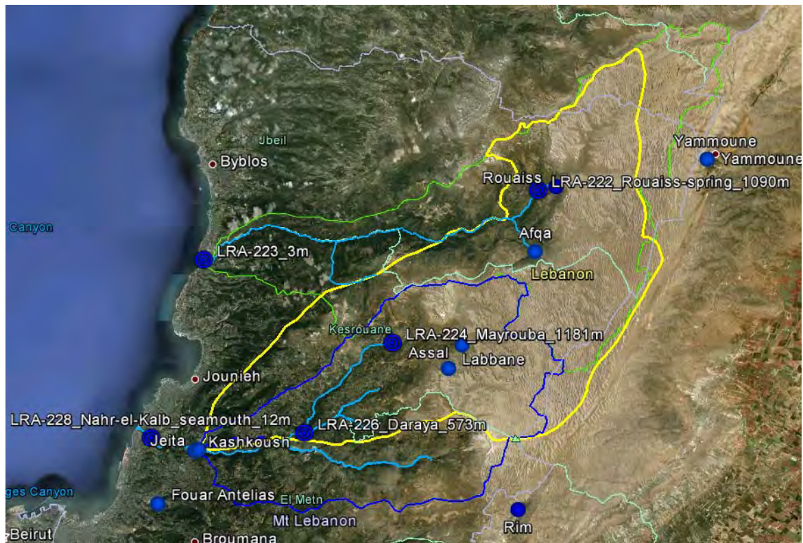
Figure 11: Stream flow gauging stations monitored by LRA in the Nahr el Kalb and Nahr Ibrahim surface water catchments
