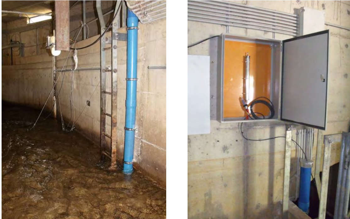
Figure 66: BGR Monitoring of Kashkoush Spring Water Quality and Discharge (data can be sent via telemetric transfer to Dbayeh treatment plant for quality control and discharge management)
