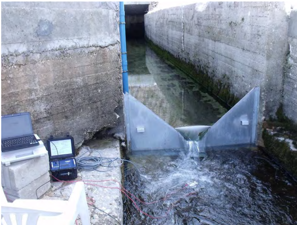
Figure 64: Triangular metal weir (120°) destroyed in May 2011 by farmers from Kfar Debbiane - measurement of tracer arrival using an Albillia fluorometer
