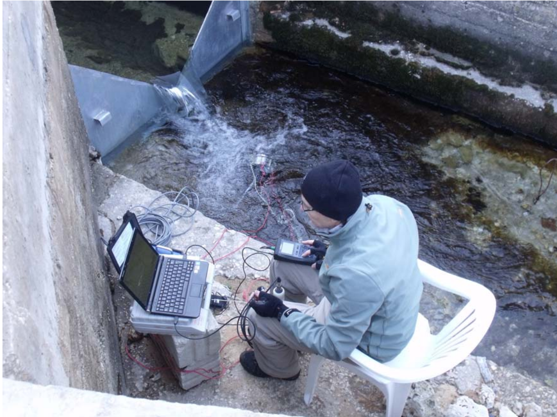
Figure 11: Flow measurements at Labbane Spring using Uranine and Salt
