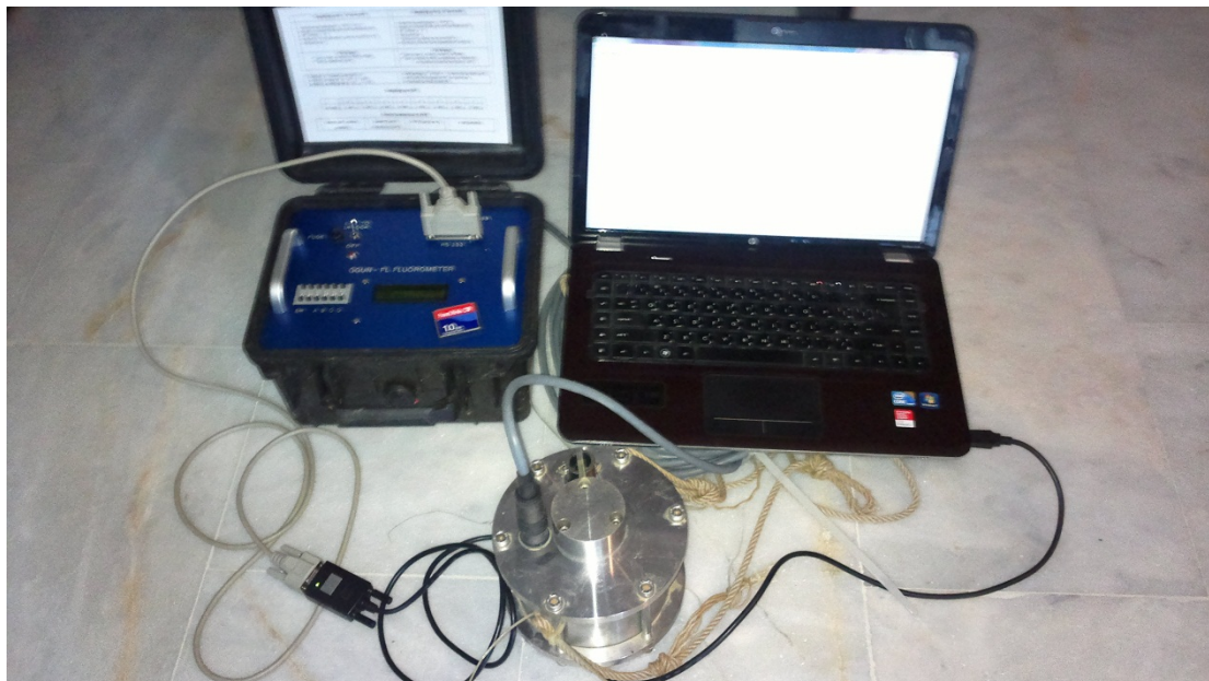
Figure 3: Equipment needed for Time Synchronization
