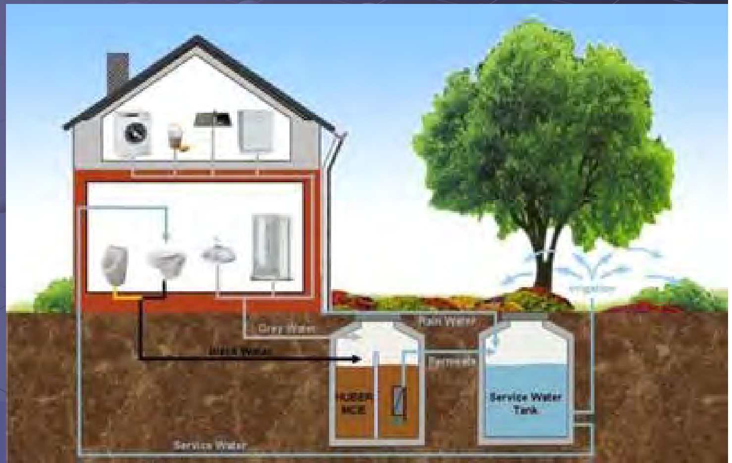
Decentralized treatment system for a single house
