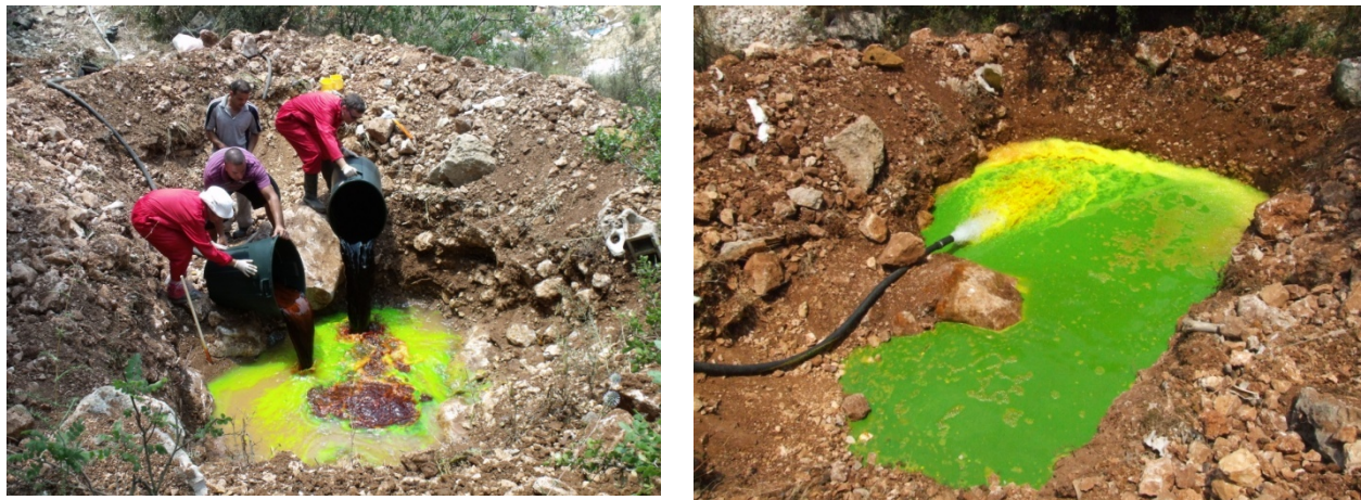
Figure 2-2 Injection of 10 kg of Na-Naphtionate and Fluorescein into the Ajaltoun artificially dug hole
