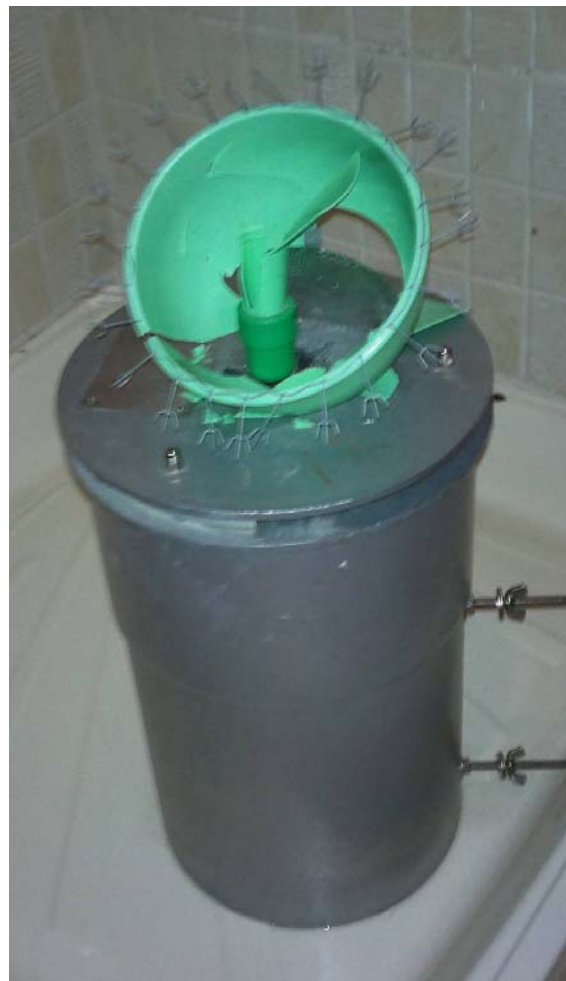
Figure 48: Damaged Funnel and Device to refuse Birds due to a Piece of Ice falling on the Instrument
