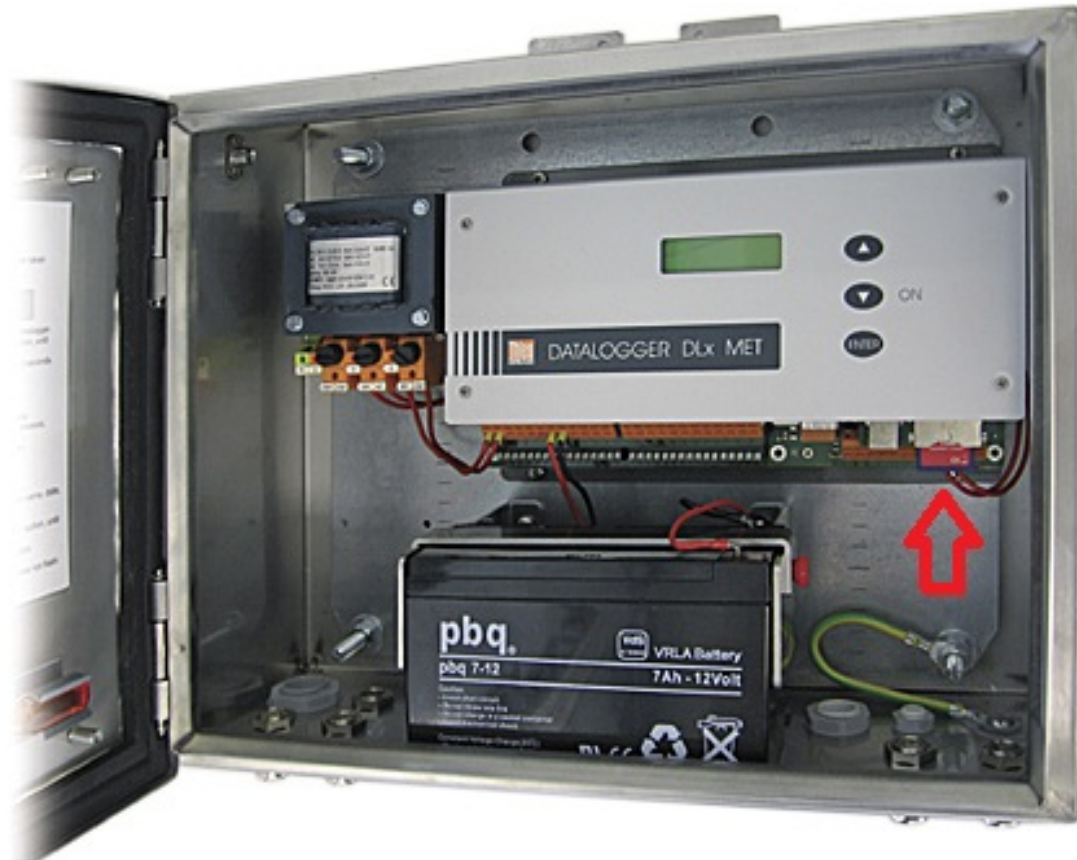
Figure 18: Datalogger DLx Met showing buttons <▼> <▲> and <Enter>, the red arrow showing the SD-Card slot.
