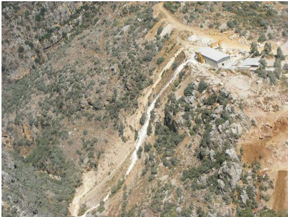
Figure 79: White sludge and waste dumped from rock cutting factory into river course, Deir Chamra
