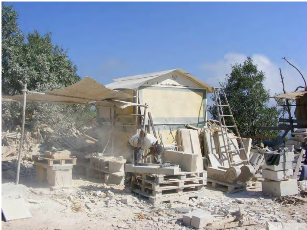
Figure 73: Rock saw at Raachine cutting decoration stone
