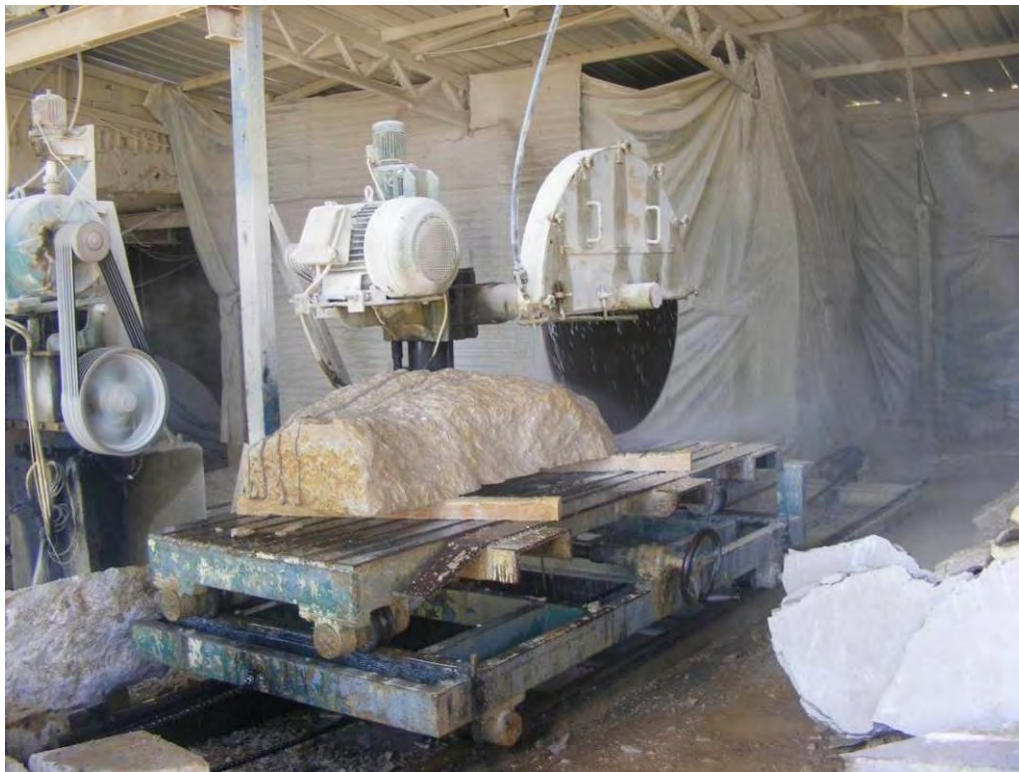
Figure 74: The rocks are cut using water with the blade to avoid dust spread in the air and related disturbances to workers
