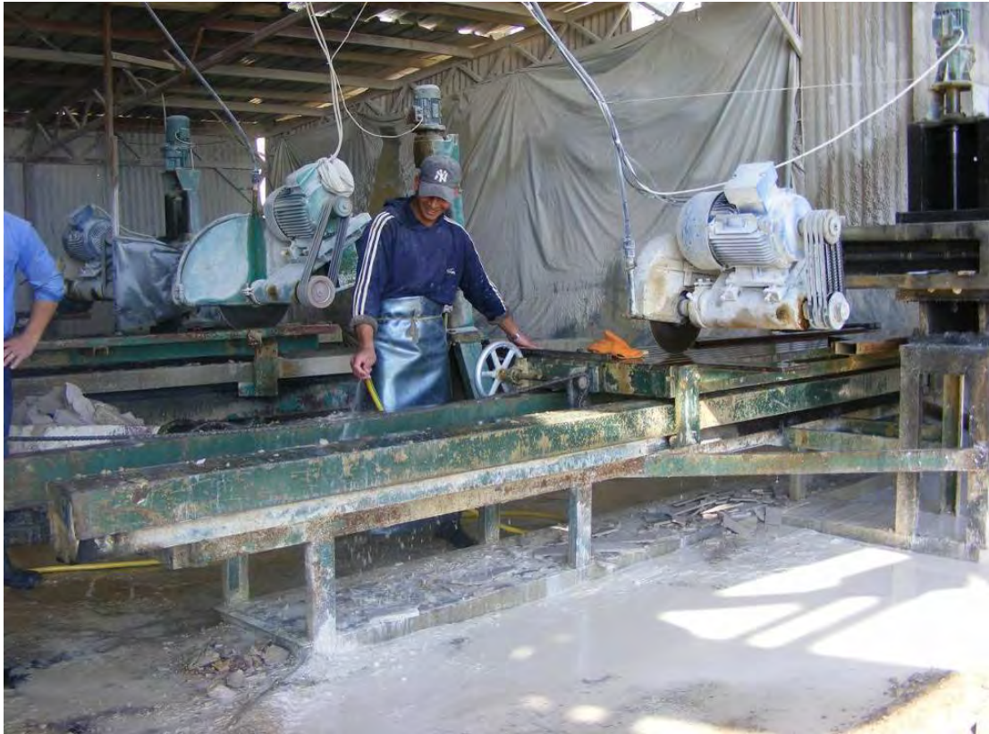
Figure 76: Cleaning of rock cutting equipment needs large amounts of water leaving fine white sludge everywhere
