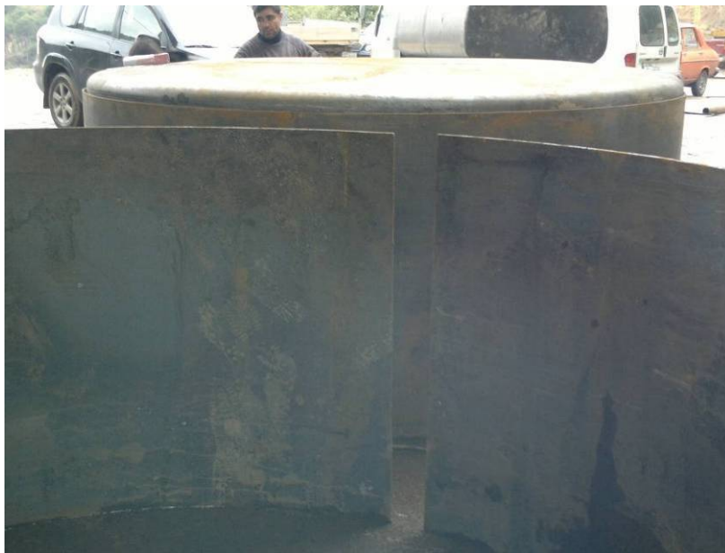
Figure 16: Carbon steel plates cut at the required length,
