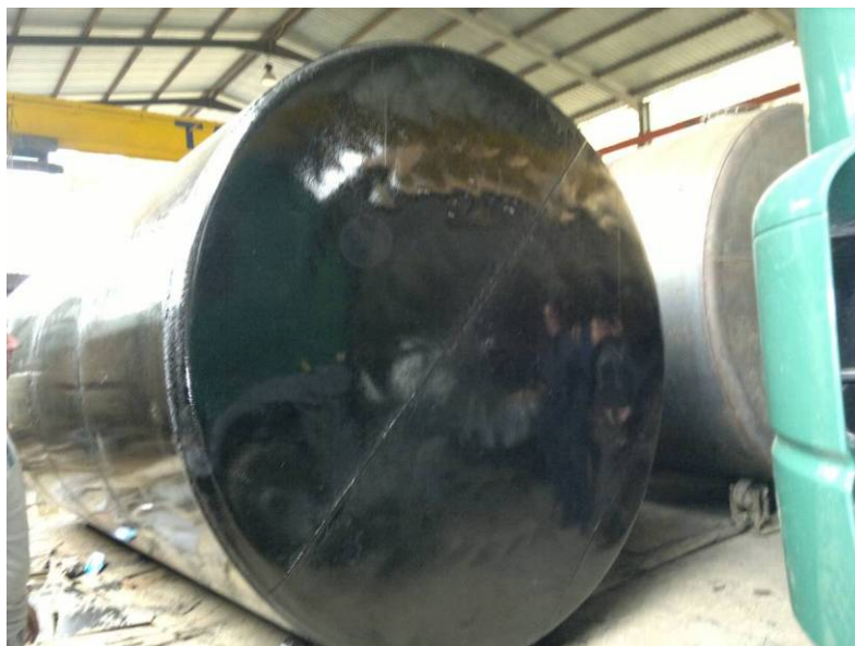
Figure 14: Two fuel storage tanks, one covered by bitumen while the other is not covered yet.
