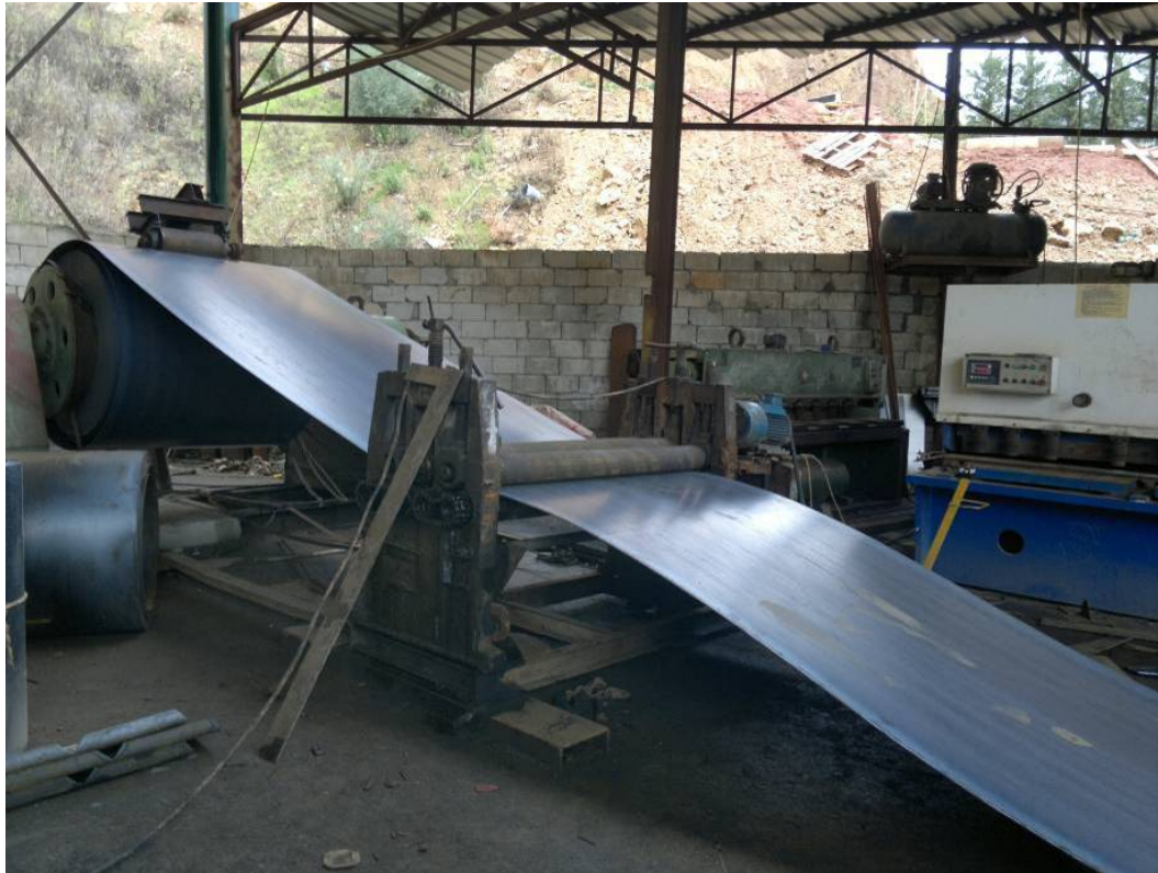
Figure 15: Roll of carbon steel plates to be cut at the required length.
