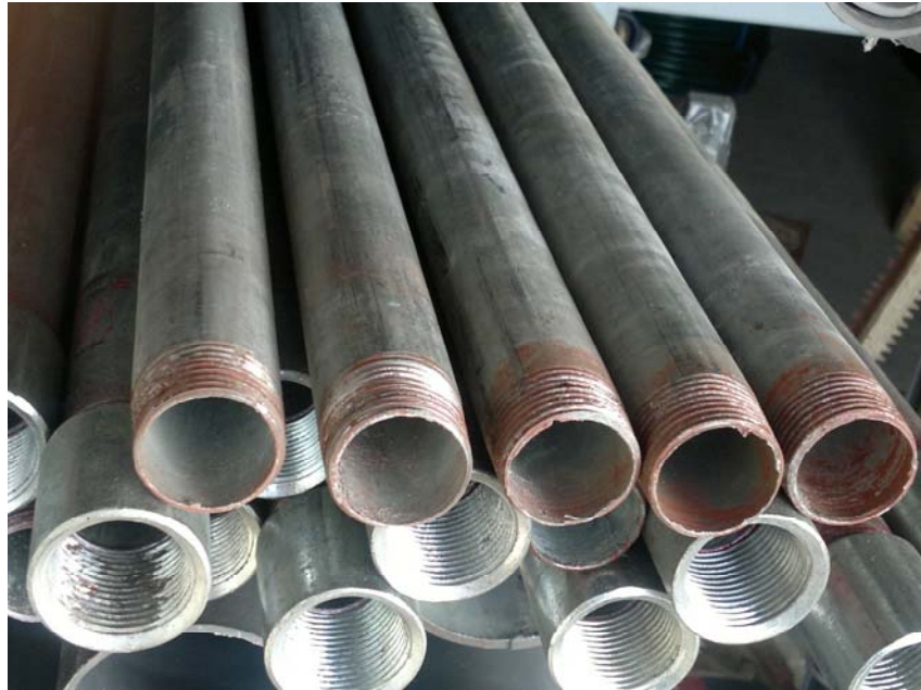
Photo 11: Uncoated pipes commonly used in gas stations in Lebanon, leading to frequent breaks and fuel leakages.
