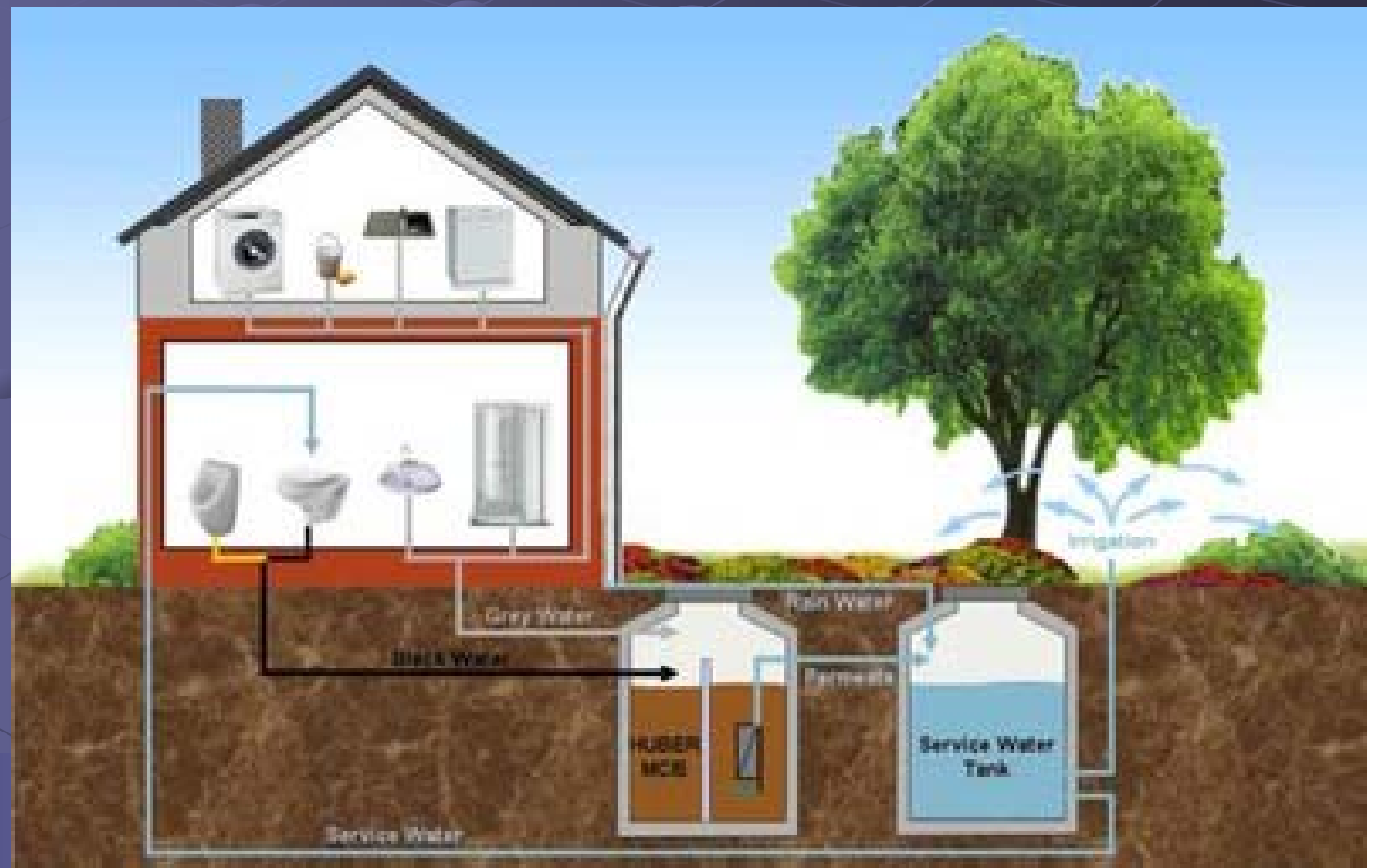
Decentralized treatment system for a single house
