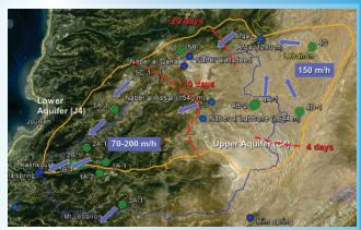
Tracertests have shown that flow velocities in the GW catchment are very high, resulting in insufficient time for attenuation of contaminants. Because the karst is directly exposed and not covered with a sufficiently thick soil, contaminants can infiltrate unhindered. The contamination risk is therefore extremely high.
