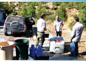
Tracertests (colorations) were done to investigate the boundaries of the groundwater catchment and the behavior of the GW system. By injecting tracer at the proposed WWTP sites it can be determined whether the effluent would arrive at a drinking water source.
