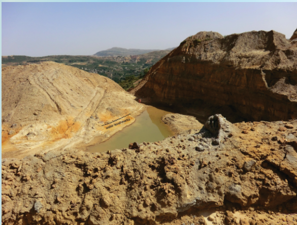
Ponds, containing silt, clay and sand are released to dispose these tailings - increasing the turbidity in affected surface waters.
