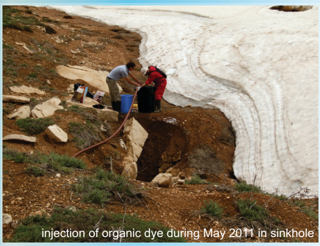
The high plateau (Upper Cretaceous limestone) is highly karstified. There are more than 2000 dolinas, where groundwater directly infiltrates. Groundwater flow is very rapid here.
