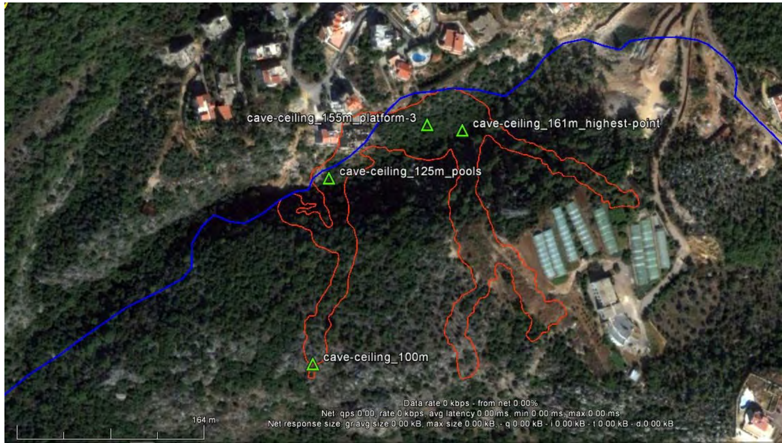
Figure 3: Superposition of Jeita cave upper level, underground river and satellite map in Google Earth
